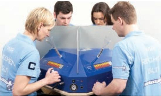
odour measurements, it is necessary to highlight the need for consistent smelling. Even evaluation from the smelling strip has to be learned and trained. To facilitate consistent smelling, Odournet GmbH has developed the PureSniff device. This is an instrument which presents the headspace over a sample in undiluted form when a panelist activates a switch. It is a universal tool for preparing and presenting the headspace and thus presents the scent of a product in its pure form.
